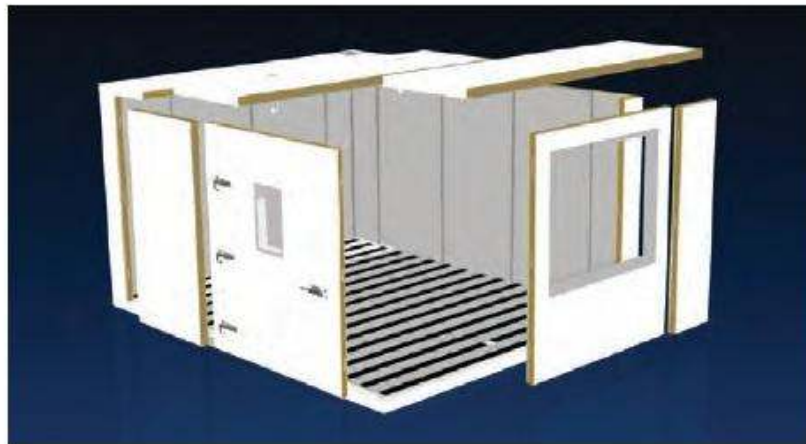
panels are easy to move in and asseble. Tongue and groove assembly is held together fixed in each other by press fit technique and sealed using silicon sealant.
